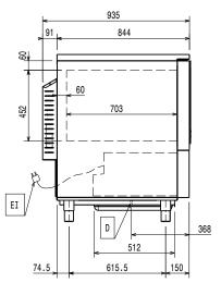
Drain Electrical inlet (power)
